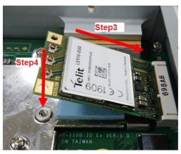
$\ensuremath{\mathbf{STEP}}\xspace\, \mathbf{5} :$  Secure the wireless module card with the 2 screws included in the package.
