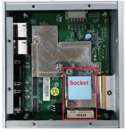
**STEP 3**: Insert the wireless module into the socket at an angle.
